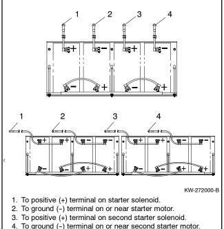
4. To ground (-) terminal on or near second starter motor.
